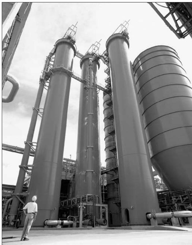
**Figure 2.6 Bleaching towers in a Kraft Mill System.** *The sulphate process, also called the Kraft pulp process, is a recovery process, where the chemicals used in the cooking of the pulp are, generally, recycled. In addition so-called black liquor produced in the process may be incinerated and as such provide the industry with all energy needed. (Photo: © Andritz AG)*
