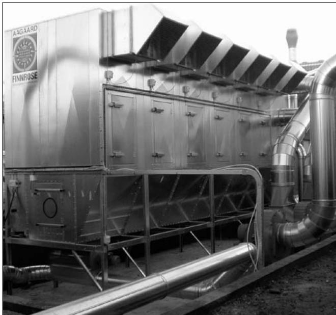
**Figure 2.1** Sleeve filters air-cleaning system AAGAARD. Produced in Denmark, in 2001.
